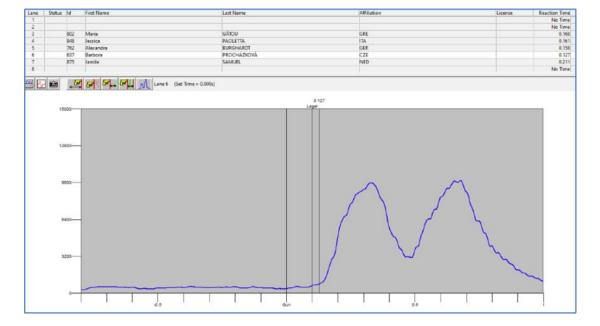
Figure 3: Start Output – reaction time and wave form lane 6 with trembling (source: MATSPORT)
